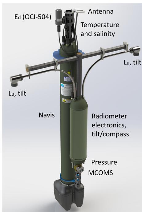
The radiometer attached to a Navis float. An OCI-504 is mounted on the mast. The two Lu heads are at the ends of the arms. An MCOMS is at the base of the housing. Carbon fiber tubes rigidly support the arms.
