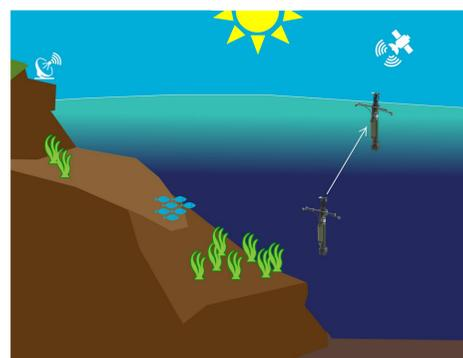
The float will park at 1000m to inhibit biofouling. On ascent, data will be collected from 300m to the surface (radiometers <0.5m), with frame rate increasing near the surface. The data collection schedule can be reprogrammed from shore.
