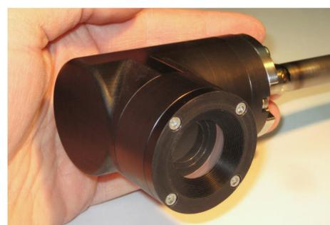
Close up of the radiometer head prototype. The head includes a shutter and tilt sensor.
